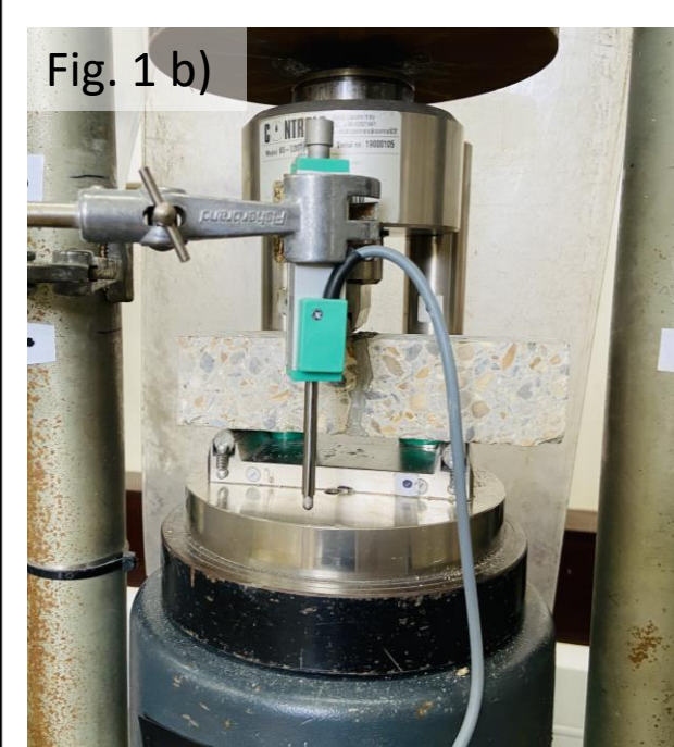
Fig. 1. Mechanical testing of enhanced repair materials: a) Commercial repair materials; a) Flexural test to measure the flexural (bending) strength, properties of the materials; and b) Plot showing the flexural properties of representative materials composed of Rapid Set and fibre additions.
