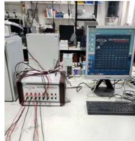
Fig 4. Rapid chloride penetration test (RCPT) set-up
