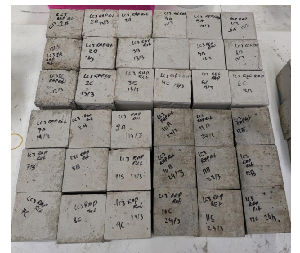
Figure 4. LC3-based rigid pavement containing 100% RAP
