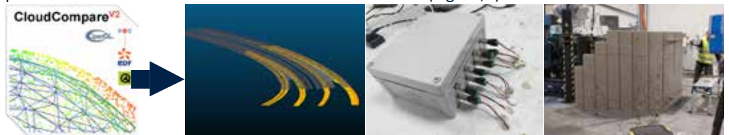
Fig. 3. a) CloudCompare to register GPR with point cloud data. b) In-house PZT sensor system and (c) Instrumented 3D printed headwall.
