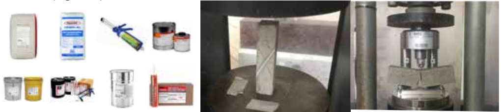
Fig. 1a) Eight selected commercial repair materials. b,c) Mechanical tests (b) Slant shear test and (c) flexural test.
